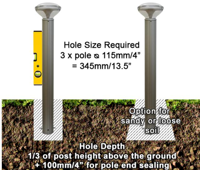
**STEP 2** - Pour concrete into the hole
